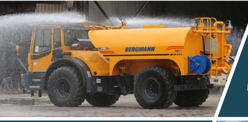
SELF-LOADING CAPABILITY AND REAR MOUNTED HOSE REEL
